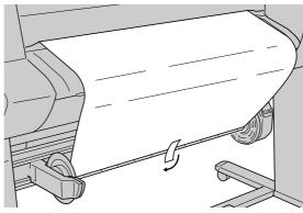
**10** Press  $\checkmark$  to feed some slack into the roll media.
